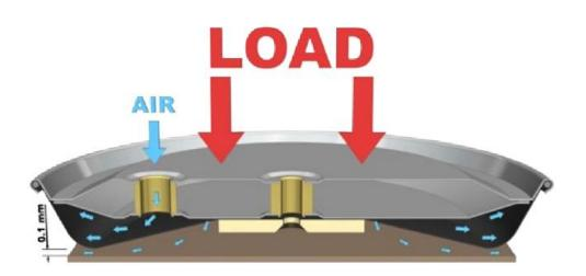
Air Casters, Air Bearings, Air Skates, they are all terms for the same thing. They are pneumatic elements that can be placed underneath an object or frame, allowing almost friction free movement and positioning in all horizontal directions.
