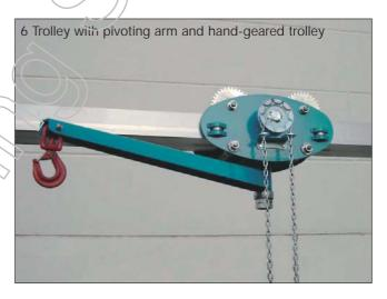
The travelling crane is designed for indoor operation. The beam consists of an aluminium section. The rest of the construction is made of painted steel. The weight of the hoist may not exceed 20 kg.
