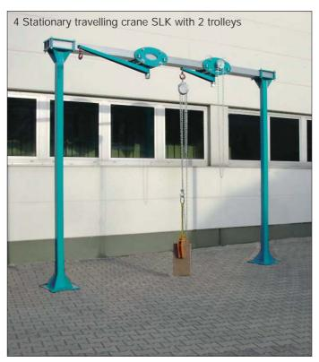
The stationary travelling crane SLK is a simple frame system. The trolley with pivoting arm covers a large working area.
