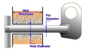
Rotate pin 180° for quick release
