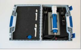
All smooth/rough and air-tight plates like tiles, natural stone- or concrete plates, plastics, metal plates or glass can be lifted easily: immediately after the Levator is positioned, it attaches itself securely to the plate and the load can be easily lifted and handled. The Levator releases the plate, when required: press the button and the valve opens. Wall tiles can also be rotated vertically.
