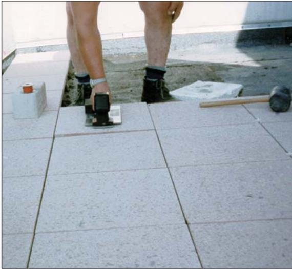
All smooth/rough and air-tight plates, e.g. tiles, natural stone or concrete plates, plastics, metal plates or glass, can be lifted easily: immediately after the Levator is positioned, it attaches itself securely to the plate and the plate can be lifted easily and handled. The Levator releases the plate, when required: press the button and the valve opens.
