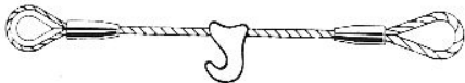
AHS 4 THIMBLE EYE ONE END, SOFT EYE OTHER END FITTED WITH CHOKER HOOK
