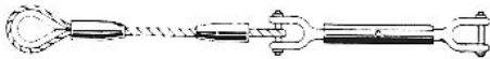
AHS 8 THIMBLE EYE ONE END, SOFT EYE AND RIGGING SCREW OTHER END
