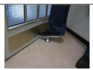
Lifts, lowers and swivels to enable smooth foot control when fitting a door. Available in two sizes:
