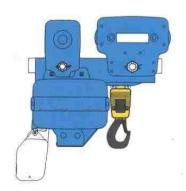
The hoist load hook is situated to one side of the hoist body to offer an increased height of lift.
