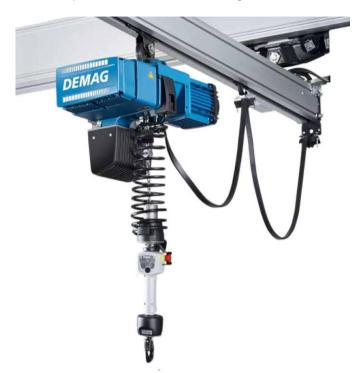
The Demag Balancer uses a standard variable speed electric chain hoist in conjunction with weight sensing and an intuitive control for precise positioning using light manual input only.
