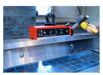
Excellent performance to weight ratio achieved by using highenergy neodymium magnets arranged in an efficient magnetic circuit. Superb holding force for a safe, reliable lift.
