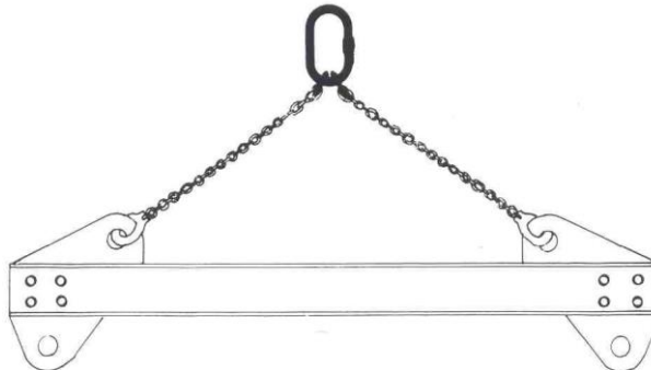
Two point pick up with a 2-leg sling suspension at each end
